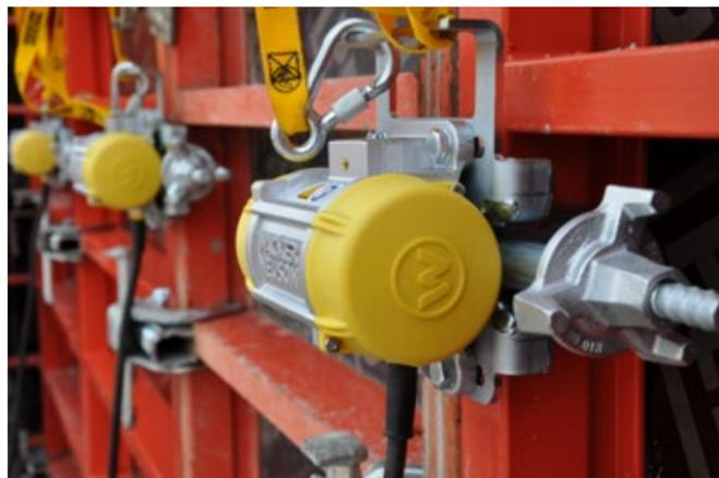
**Flexible for in-situ concrete applications.** There is a large selection of fastening clamps available from Wacker Neuson for the AR26. These can be attached to all common formwork.
