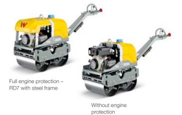
The variable protective frame concept gives the greatest possible flexibility, for different requirements and applications.
