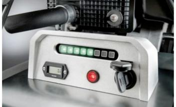
Compatec compaction display: It indicates when the maximum compaction has been achieved with the unit. Learn more at: www.wackerneuson.com/compatec
