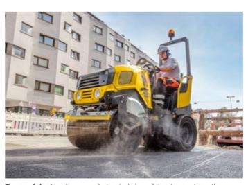
Tapered design: for an unobstructed view of the drum edges, the machine surroundings and the construction site.
