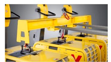
Flexible lifting: the lifting beam can be used both for the 2-unit and for the 3-unit coupling set.
