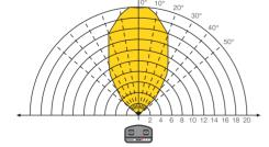
Far-reaching control: A transmission field of up to 20 meters and an angle of 45° guarantee a high level of working comfort.
