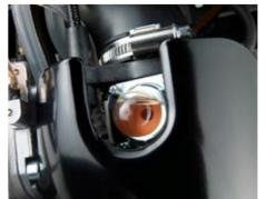
Feed pump at the carburetor – for full and immediate power of the WM80.
