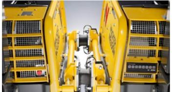
**Stable coupling**: quickly and reliably connected with a few screws.
