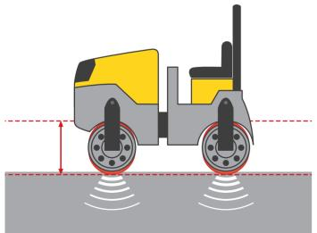
Both the vibration drums optimally bring the material to be compacted optimal oscillation with quick successive vertical forces.
